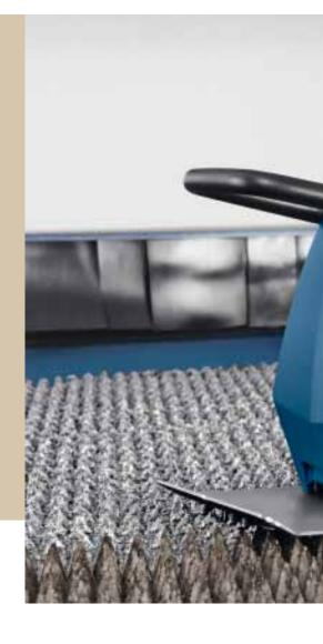
If you cut sheet metal with a flatbed laser machine, now you can save up to 75% of the cost of support slats. The TRUMPF TruTool TSC 100 slat cleaner cleans slag from your slats – over and over, and much more quickly than cleaning by hand. So you can use your support slats significantly longer.
