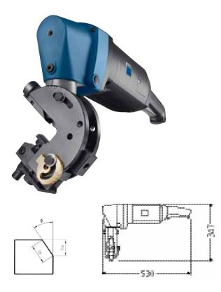
Bevelling angle easily adjustable from 20° to 55° Processes pipe with a minimum inside diameter of 30 mm Roller guide reduces vibration for comfortable machining and longer cutter life Processing of T- and double T-carriers
