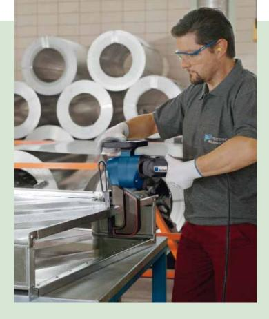
Whether in HVAC or in container and equipment construction, joining is probably the simplest and most cost-effective way to connect two metal parts. The TRUMPF power fastener uses a unique cold-forming technology to punch a small dimple into both sheets and immediately you have an astonishingly stable, long-lasting connection. No screws, no rivets, no emissions, no preparation or cleanup work.
